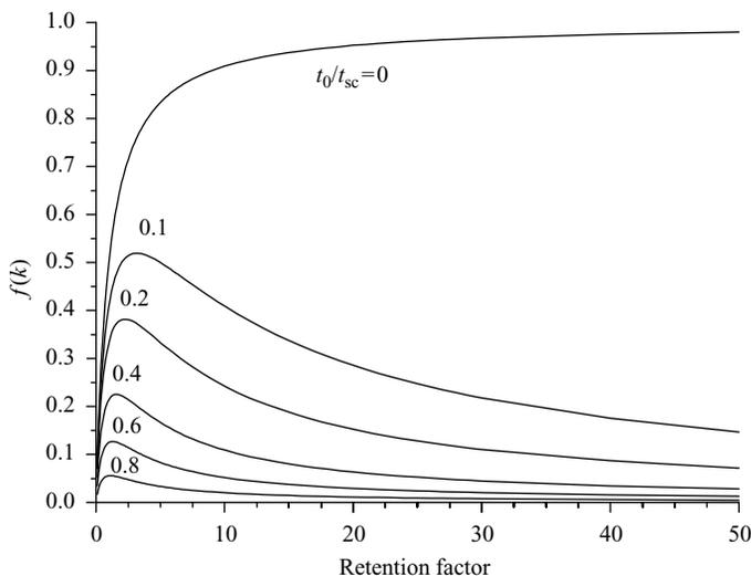
**Figure 1.6** Dependence of  $f(k)$  on the retention factor in EKC in the normal elution mode [see Equation (1.13)] for several ratios  $t_0/t_{sc}$ . The ratio  $t_0/t_{sc} = 0$  corresponds to conventional chromatography with an immobilized stationary phase (according to [12])
