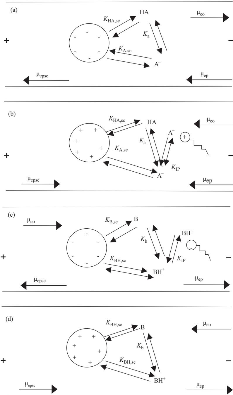
**Figure 1.8** Interaction of ionizable solutes with micellar separation carriers: (a) acidic solute (AH) with anionic SC; (b) acidic solute (AH) with cationic SC; (c) basic solute (B) with anionic SC; (d) basic solute (B) with cationic SC (according to [74])
