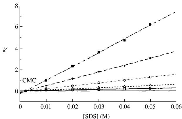
**Figure 1.5** Dependence of the retention factor  $k'$  for several neutral solutes on the molar concentration of the anionic surfactant SDS in the separation buffer; solutes: ■ 2-naphthol, \* toluene, ○ nitrobenzene, △ phenol, □ resorcinol. (Reprinted with permission from M.G. Khaledi, S.C. Smith, J.K. Strasters, *Anal. Chem.*, **63**, 1820–1830 (1991), copyright 1991 American Chemical Society)
