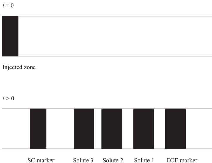
**Figure 1.4** Development of solute zones during the chromatographic run, normal elution mode, neutral solutes,  $P(\text{Solute 1}) < P(\text{Solute 2}) < P(\text{Solute 3})$  [see Equation (1.5)]
