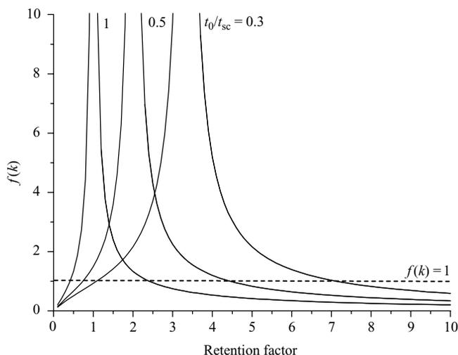
**Figure 1.7** Dependence of  $f(k)$  on the retention factor in EKC in the restricted elution mode [left side of the graph, see Equation (1.15)] and the reversed migration mode [right side of the graph, see Equation (1.14)] for several ratios  $t_0/t_{sc}$ . The dashed line indicates  $f(k) = 1$  (according to [21])
