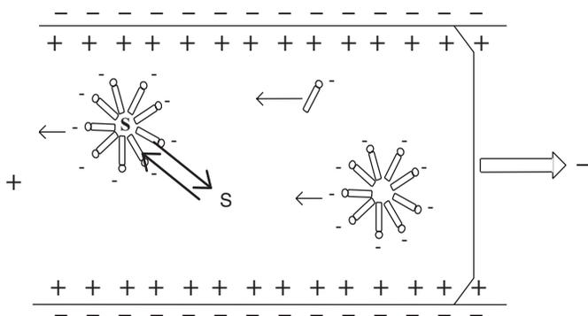
**Figure 1.1** Scheme illustrating the separation mechanism in micellar EKC (anionic surfactant, normal elution mode)
