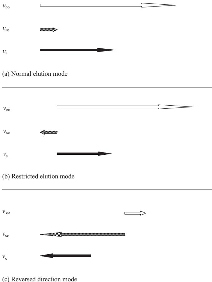
**Figure 1.3** Elution modes in electrokinetic chromatography
