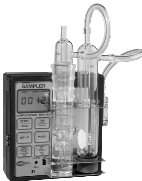
Figure 1.7. Midget impingers collect air contaminants in a liquid for later laboratory analysis. (Courtesy of SKC, Inc.)
