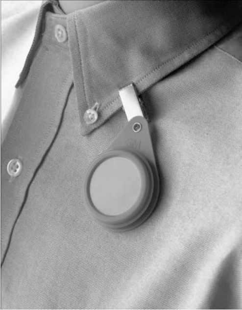
Figure 1.3. Passive dosimeter collects gases and vapors without a sampling pump. (Courtesy of SKC, Inc.)
