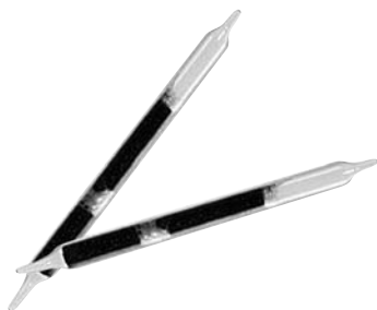
Figure 1.6. Charcoal adsorption tubes collect organic vapor for later laboratory analysis. (Courtesy of SKC, Inc.)
