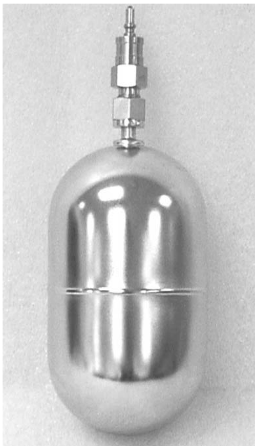
Figure 1.5. Evacuated cylinders collect samples at a controlled rate without use of a pump. They are available in a variety of sizes. (Courtesy of Galson Laboratories.)
