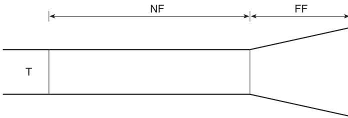
Figure 1.6a This diagram shows the shape of the unfocused ultrasound beam as it emerges from the transducer with a narrow near field (NF) and a diverging far field (FF).
