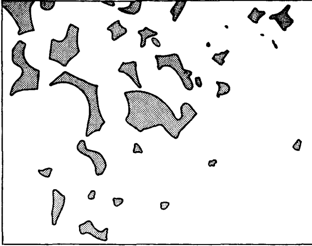
Fig. 1.3 Simplified pore space (black) in a section of smacked carbonate rock.
