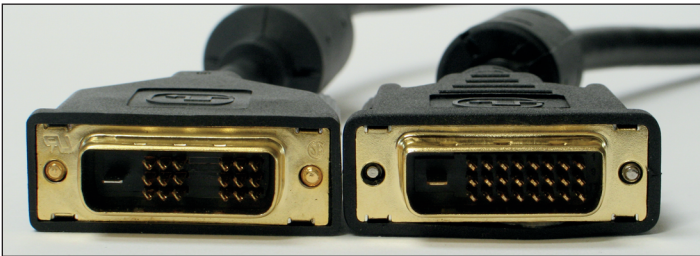
1.3 DVI-D single-link (left) and dual-link (right) connectors.
