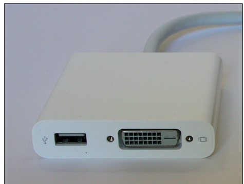
1.5 Use the Apple Mini DisplayPort to Dual-Link DVI adapter to connect your Mac's Mini DisplayPort to an external display's dual-link DVI port.
