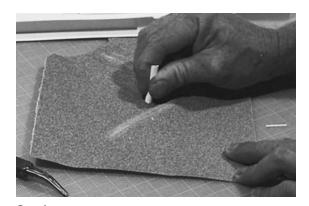
**Sandpaper** Sandpaper can be used to level and remove the burrs from cuts.
