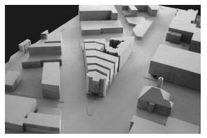
**Massing model** Small massing models are typical of the building representations used for site plans.
