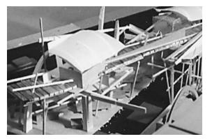
**Plastic Mylar** Mylar drafting sheets can be easily cut and used for curved translucent panels.
