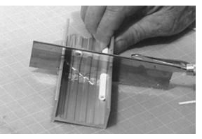
**Modeling Saw and Miter Box** Used for clean cuts on small blocks and rods as well as angle cuts.
