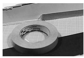
**Double-Face Transfer Tape** Used to attach paper without the buckling tendencies of white glue.
