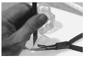
Acetate Adhesive Used for Plexiglas. A drop on the end of a knife blade can be applied by dragging the blade along the edge of the Plexiglas.
