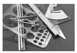
**Drafting Tools** A set of common drawing tools used to lay out the model parts.
