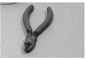
**Side Cutters** For cutting pins and wire.
