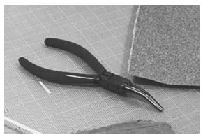
**Needle-Nose Pliers** Used for delicate work and as an inexpensive third hand.
