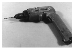
**Electric Drill and Small Bits** Used for gang-drilling multistory column holes in floor plates and other special holes.
