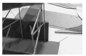
**Small Plastic Triangle** Used to square and level model parts for accurate assembly.
