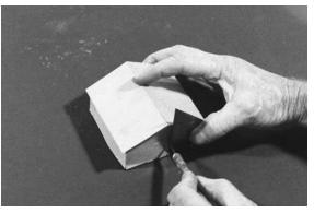
**Small Metal and Plastic Triangles** Can be used to align model parts for gluing and for making accurate modification cuts directly on the model.
