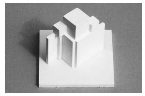
**Massing model** The kind of block massing typical of models that reflect only the solid form of the building.
