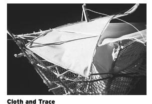
Drawing trace or light cloth can be used to fill in planes and simulate translucent membranes. These materials can be curved and warped as needed.
