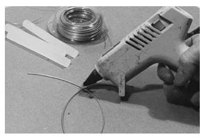
**Hot Glue Gun** For quick assembly and hard-to-glue materials like metal. Can be very messy and is not well suited for finish work.
