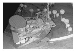
**Metal Sheets** Thin metal sheets can be used to make planes and curving forms (see Chapter 5).
