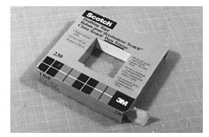
**Drafting Tape** Used to attach parts while glue is setting. Avoid masking tape, as it will tear paper surfaces.
