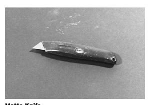
**Matte Knife** For cutting very thick materials. The blade thickness on this tool is not suited for fine work.
