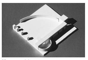
**Diagram model** Diagrams can be used to explore basic organizational schemes such as a datum wall to set up overall relationships.
