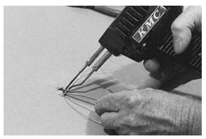
**Soldering Gun** For soldering copper and steel wire. *Note:* Use rosin-core solder.
