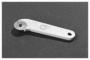
**Rolling-Style Pizza Cutter** Used for transferring drawing lines to modeling surfaces. Roll cutter along lines to leave traces in modeling material. Cutters with pointed edges work best.
