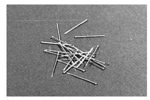
**Straight Pins** Used to attach parts while glue is setting. Pins can be pulled, set for reinforcement, or cut off with side cutters.
