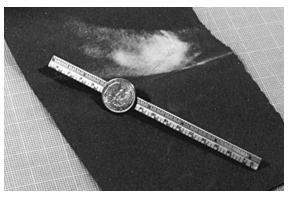
**Small-Scale rule with End Cut Off** Used for taking measurements directly from the model. A scale can be drawn on a wooden stick to serve the same purpose.
