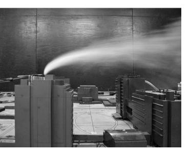
For this detailed study of wind-wake analysis at the University of Colorado Denver's new Research 1 and 2 complexes in Aurora, Colorado, computer simulation or physical wind-tunnel testing can ensure that exhaust streams will be safely dispersed and diluted before getting to nearby buildings, out-door occupant areas, or air intake louvers in the vicinity. *Image courtesy of RWDI*.
